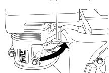
Figure 19 - Choke Lever Opened (Model PGH7500IE Shown)
